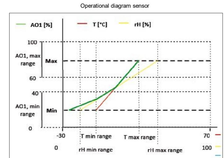
Note: The output changes automatically depending on the highest T or rH values, i.e. the highest of the three output values controls the output. See the green line in the operational diagram above.
