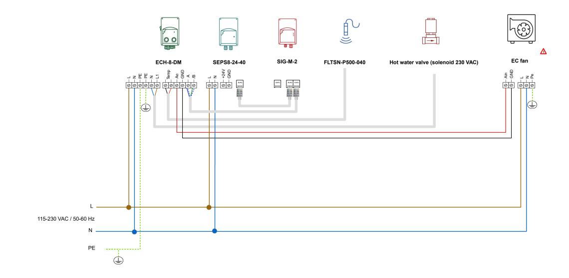
Consult the fan manufacturer for the correct wiring. First connect the products, then download the firmware for this solution ID via SenteraWeb. The firmware will be automatically downloaded in the connected device(s).
