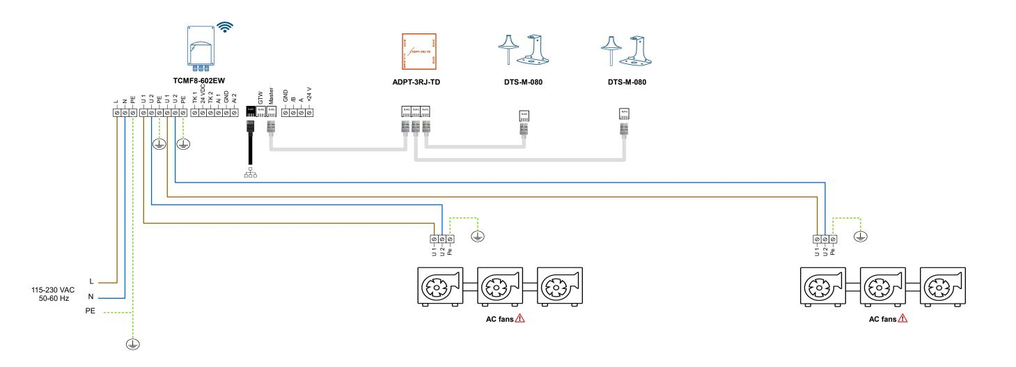
Consult the fan manufacturer for the correct wiring. First connect the products, then download the firmware for this solution ID via SenteraWeb. The firmware will be automatically downloaded in the connected device(s).
