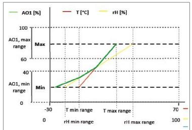
Note: The output changes automatically depending on the highest T or rH values, i.e. the highest of the three output values controls the output. See the green line in the operational diagram above.
