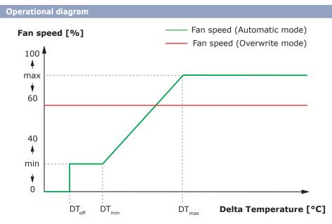
The smaller the difference between  $DT_{min}$  and  $DT_{max'}$  the faster the fan speed will be adjusted. If the ceiling fans speed up too fast, increase the difference between  $DT_{min}$  and  $DT_{max}$  to make the ceiling fans accelerate slower.
