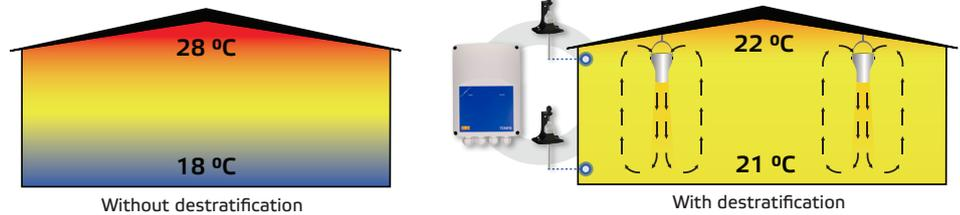
When the difference between ceiling and floor temperature is lower than  $DT_{OFF}$ , the fans are disabled.
