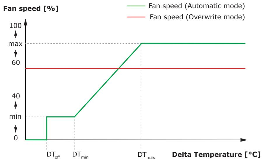
The smaller the difference between  $DT_{min}$  and  $DT_{max}$ , the faster the fan speed will be adjusted. If the ceiling fans speed up too fast, increase the difference between  $DT_{min}$  and  $DT_{max}$  to make the ceiling fans accelerate slower.
