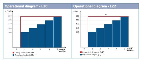
The unregulated output is active when the air curtain is enabled. Because this output is either ON (230 Volt) or OFF (0 Volt), it is called 'unregulated output'. The maximum current of this output is 2 A. It can be used to control a water valve to regulate the flow of hot water to the LPHW coil.
