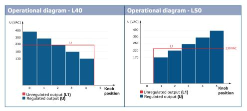
The unregulated output is active when the air curtain is enabled. Because this output is either ON (230 Volt) or OFF (0 Volt), it is called 'unregulated output'. The maximum current of this output is 2 A. It can be used to control a water valve to regulate the flow of hot water to the LPHW coil.
