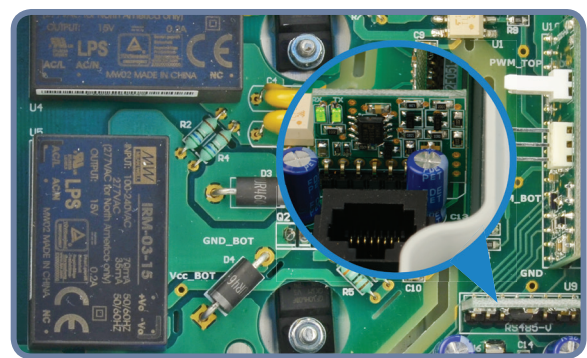
Fig. 8 Communication LED indication
