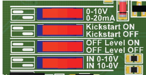
Fig. 4 DIP switch settings
