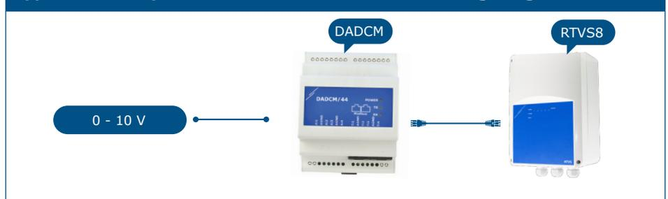
**Application example 4: Automatic mode - control via a digital potentiometer**
