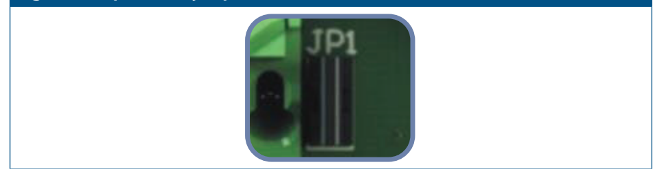
Fig. 4 Pull-up resistor jumper 1
