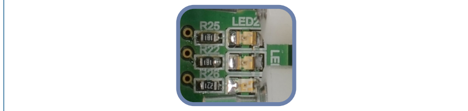
Fig. 5 LED indication connection to the Internet
