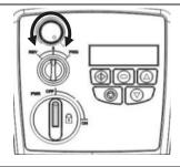
The potentiometer will control the motor shaft rotational speed.
