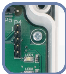
Fig. 9 Modbus holding register reset jumper
