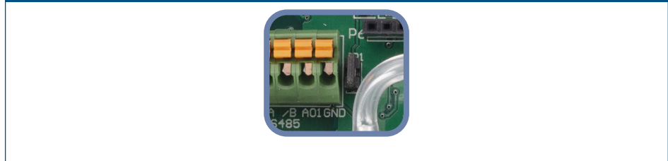
Fig. 5 Pull-up resistor jumper connected
