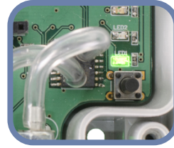
Fig. 16 Power / Modbus communication indication
