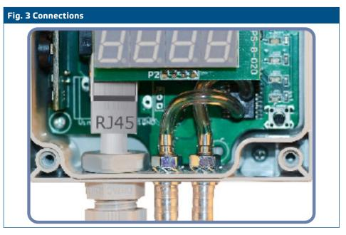
5. Connect the nozzles to the duct (see Fig. 4). Depending the application you must use a specific connection set to connect the nozzles of the unit to the duct:
