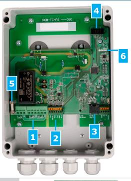
1 - Terminal block power supply and regulated outputs
