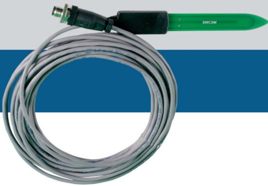
SWCSM-075 is a soil water content sensor equipped with a digital temperature sensor. It is supplied with 24 VDC Power over Modbus. The measured values and all other parameters are accessible via Modbus RTU.
