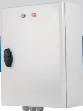
The STVS4 series of transformer fan speed controllers regulate the rotational speed of three-phase voltage controllable motors in five steps by varying the output voltage according to a 0–10 VDC analogue input signal. They are equipped with auto-transformers and feature TK monitoring for thermal motor protection.
