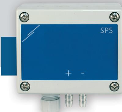
The SPS2 differential pressure controller controls directly EC fans, frequency inverters or other control units with two differential pressure setpoints (high/low or day/night mode option). It provides an analog or digital output with integrated PI control and K-factor setting. The two setpoints can be switched via external switch / contact or digitally. All system parameters are controllable via Modbus RTU communication.
