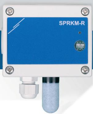
The SPRKM-R are multifunctional parking garages gas sensors which measure temperature, relative humidity, CO and LPG (propane C<sub>3</sub>H<sub>8</sub>) levels. They are Power over Modbus supplied and all parameters and the output value are accessible via Modbus RTU.
