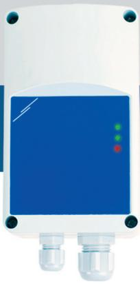
SIG-M-2 is an internet gateway to connect a stand-alone Sentera device or a network of devices to the Internet in order to configure or monitor them via SenteraWeb. The SIG-M-2 makes wireless or wired connection with the internet router. The unit has 2 Modbus RTU channels - a Master channel to communicate with the connected Slave devices, and a Slave channel to make the unit accessible for a Master controller or a BMS.
