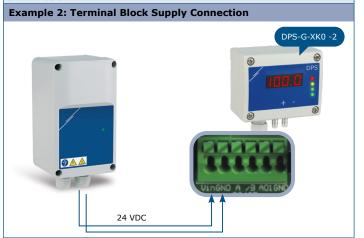
In this example, SEPS8 is connected to a differential pressure transmitter from the DPS-G-XKO -2 series through terminal block supply connection, which provides 24
