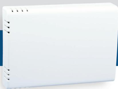
The RXC series are room sensors / switches which measure the concentration of CO<sub>2</sub> in the air. Four pre-defined ranges provide ideal measurement windows with one user-definable range. The implemented sensor is self-calibrating and maintenance-free. These units are equipped with Modbus RTU (RS485) communication and have an analog output and a relay output.
