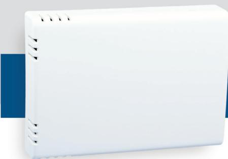
The RXC series are room sensors / switches which measure the concentration of CO<sub>2</sub> in the air. Four pre-defined ranges provide ideal measurement windows with one user-definable range. The implemented sensor is self-calibrating and maintenance-free. These units are equipped with Modbus RTU (RS485) communication and have an analog output and a relay output.
