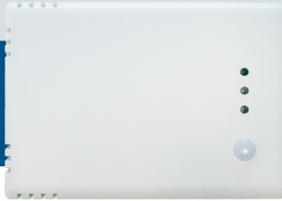
The RWTHM-2 series are combined indoor transmitters which measure indoor temperature, relative humidity and ambient light. Based on these measurements, the dew point can be calculated. They are equipped with a second temperature sensor located on an aluminium plate on the backside of the device enclosure in order to measure the temperature of the surface onto which it is mounted. The series are Power over Modbus supplied and all the parameters are accessible via Modbus RTU.
