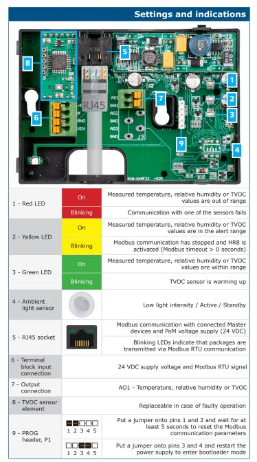
**Note:** By default, the LED indicators visualise the measured TVOC level. When the sensor is in bootloader mode, the green and yellow LEDs flash alternately. During the firmware download, the red LED is flashing additionally.
