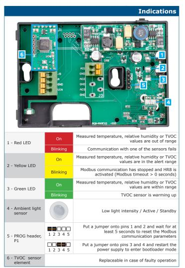
**Note:** By default, the LED indicators visualise the measured TVOC level. When the sensor is in bootloader mode, the green and yellow LEDs flash alternately. During the firmware download, the red LED is flashing additionally.
