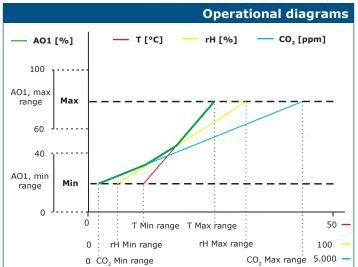
**Note:** The output changes automatically depending on the highest of the T, rH or  $CO_2$ values, i.e. the highest of the three output values controls the output. See the green line in the operational diagram above. One or multiple sensors can be deactivated. E.g. it is also possible to control the output based on the measured  ${\rm CO_2}$  value only.
