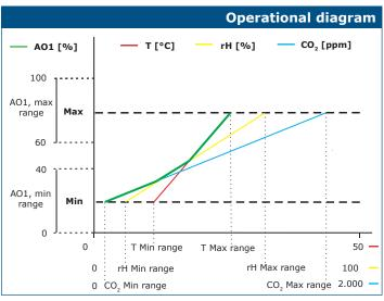
**Note:** The output changes automatically depending on the highest of the T, rH or  $CO_2$  values, i.e. the highest of the three output values controls the output. One or multiple sensors can be deactivated. E.g. it is possible to control the output based on the measured  $CO_2$  value only.
