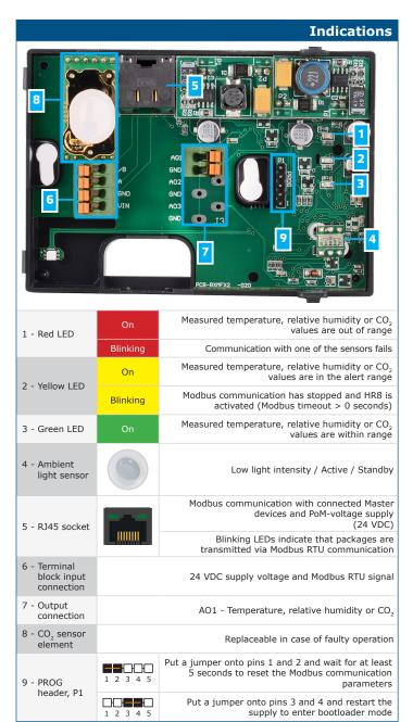
Note: By default, the LED indicators visualise the measured  ${\rm CO_2}$  level. When the sensor is in bootloader mode, the green and yellow LEDs flash alternately. During the firmware download, the red LED is flashing additionally.
