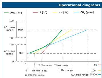
**Note:** The output changes automatically depending on the highest of the T, rH or  $CO_2$  values, i.e. the highest of the three output values controls the output. See the green line in the operational diagram above. One or multiple sensors can be deactivated. E.g. it is also possible to control the output based on the measured  $CO_2$  value only.
