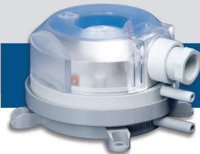
The PSW series are highly sensitive, adjustable differential pressure switches suitable for monitoring overpressure, vacuum and differential pressure of air or other non-combustible, non-aggressive gases. The switching pressure setpoint can be adjusted by means of a scaled calibrated knob; the switching  $\Delta P$  - by a screwdriver and a pressure gauge.
