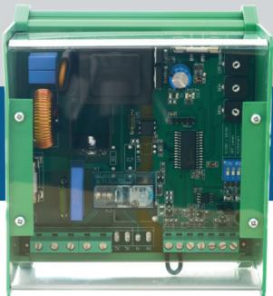
The MVS series control the speed of single-phase voltage controllable electric motors (230 VAC / 50–60 Hz) according to a standard input control signal. They are equipped with Modbus RTU communication and provide a wide range of functionalities: remote control options, adjustable off level, min. and max. output voltage settings, and time-limited motor operation initiated by a logic or switch signal.
