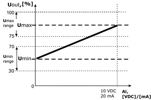
Visualisation of ascending analogue input control and off-level enabled
