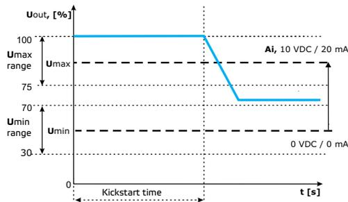
Output with kickstart and off-level enabled
