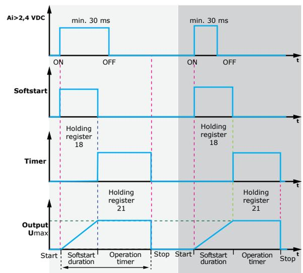
**\*Timer mode** allows the fan to operate for a predefined period, which is set via the Modbus registers of the MVS series. When Timer mode is selected in remote input function, the controller receives a pulse control signal from the remote control switch. When Timer mode is selected in analogue input function, the controller receives a pulse control signal directly from the Ai input. In both cases, the pulse width is to be more than 30 ms; otherwise, the signal is filtered (left out).
