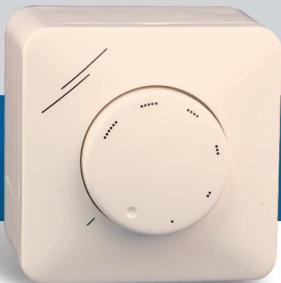
The MTV-1-010-NA potentiometer is developed to control equipment that needs a 0–10 VDC control signal. The potentiometer needs a supply of 230 VAC, and gives a stepless output signal 0–10 VDC. It is suitable for inset mounting (IP44) as well as for surface mounting (IP54).
