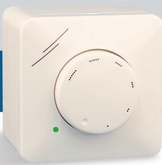
The LTV-1-010-NA potentiometer is mounted in a splash-proof enclosure. It is suitable for both inset (IP44) and surface mounting (IP54). The potentiometer needs a 230 VAC / 50–60 Hz supply and has a green LED operating indication. It provides a stepless output signal from 0–10 VDC which makes it suitable to control fans equipped with EC motor or to be used as an input device for controllers that require a 0–10 VDC control signal.
