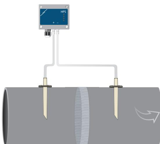
**Application 2:** Measuring supplied air volume [ $\text{m}^3/\text{h}$ ] or airflow velocity [ $\text{m}/\text{s}$ ] using PSET-PT
