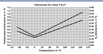
The diagram above shows the temperature and resistance tolerances for RTDs at different temperatures.
