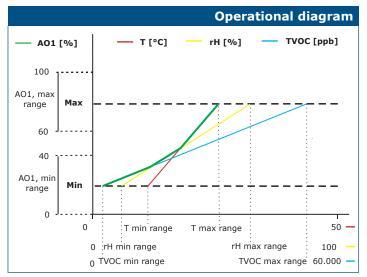
Note: TVOC measurements will return 0 ppb during warm-up time. The output changes automatically depending on the highest of the T, rH or TVOC values, i.e. the highest of the three output values controls the output. See the green line in the operational diagram above. One or multiple sensors can be deactivated. E.g. it is also possible to control the output based on the measured TVOC values only.
