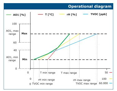
**Note:** TVOC measurements will return 0 ppb during warm-up time. The output changes automatically depending on the highest of the T, rH or TVOC values, i.e. the highest of the three output values controls the output. See the green line in the operational diagram above. One or multiple sensors can be deactivated. E.g. it is also possible to control the output based on the measured TVOC values only.
