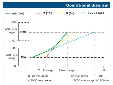
Note: TVOC measurement will return 0 ppb during warm-up time. The output changes automatically depending on the highest of the T, rH or TVOC values, i.e. the highest of three output values controls the output. See the green line in the operational diagram above. One or multiple sensors can be deactivated. E.g. it is also possible to control the output based on the measured TVOC values only.
