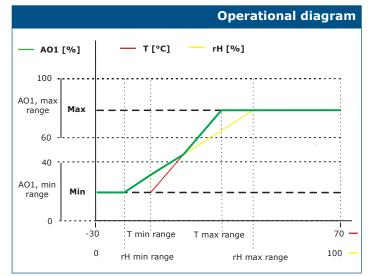
**Note:** The output changes automatically depending on the higher of the T and rH values, i.e. the higher of two output values controls the output. See the green line in the operational diagram above.
