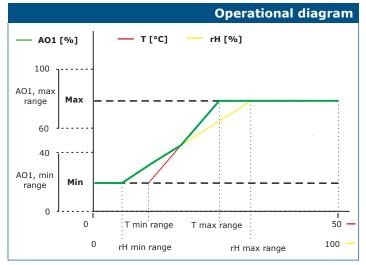
Note: The output changes automatically depending on the highest of the T or rH values, i.e. the highest of two output values controls the output. See the green line in the operational diagram above. One or multiple sensors can be deactivated. E.g. it is possible to control the output based on the measured temperature value only.
