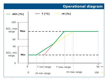
Note: The output changes automatically depending on the highest of the T or rH values, i.e. the highest of two output values controls the output. See the green line in the operational diagram above. One or multiple sensors can be deactivated. E.g. it is also possible to control the output based on the measured temperature only.
