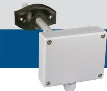
The DXTH series are dual duct transmitters / switches which measure temperature and relative humidity. For each, there are 4 pre-defined ranges acting as measurement windows plus one user-definable range. These units are equipped with Modbus RTU (RS485) communication and have an analog and a relay output for each measuring unit.
