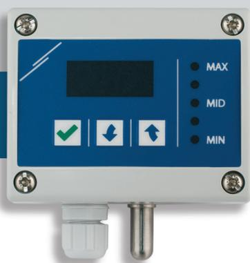
The DTAP series are universal programmable controllers. They have a temperature and/or analogue input (0–10 VDC / 0–20 mA / PWM) and provide a proportional analogue output with two setpoints, digital readout and output LED indication. The DTAP controller features programming of the setpoints for inputs and outputs.
