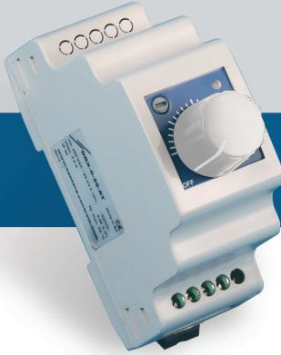
DRX and DRY series are variable speed controllers for AC fans with single-phase voltage controllable motor. They provide high to low (DRX) or low to high (DRY) output regulation and minimum output voltage adjustment. The controller enclosure is designed for mounting onto a standard 35 mm DIN rail.
