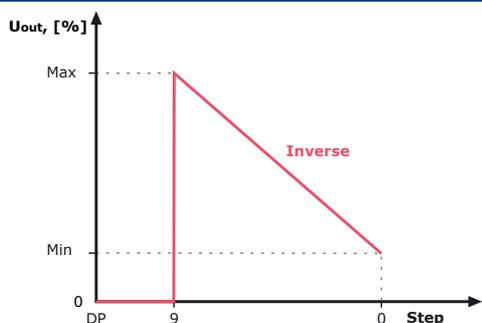
**Note:** All the diagrams refer to an ideal case of a resistive load. When using inductive loads, the output voltage might be lower depending on the inductance value! Adjust steps so that to set the required voltage.
