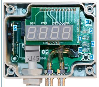
1 - Sensor calibration and Modbus register reset tactile switch (SW1)
